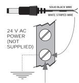
NOTE: IF ONE TERMINAL OF POWER SOURCE IS GROUNDED, HOOK THE WHITE STRIPED WIRE TO THIS TERMINAL
