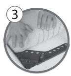
Slide a plain filter pad bunder the powerbar. © DO NOT ATTEMPT TO REMOVE POWERBAR. Place the CARBON STRINGED filter pad 3 STRING SIDE DOWN on top of and flush with the plain filter pad.
