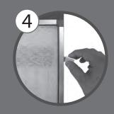
Make sure the filter pad is snug to the rails of the filter with no gaps. Close the front panel, then close both latches.
